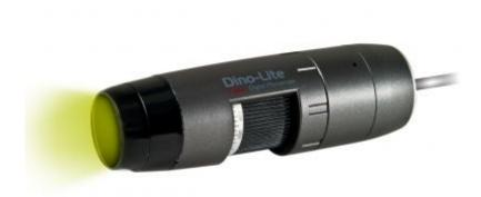
The Dino-Lite AM4115T-RFYW digital microscope is optimized for research and viewing fluorescent objects by using 575nm excitation LEDs. It has a long-pass type 610nm emission filter that is designed to observe a wide range of fluorophores with applications in developmental biology, pathology, and anatomy.
