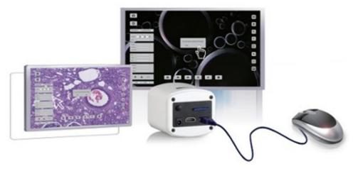
**Build-in mouse control:** the user controls the on-screen menu in HDMI mode through a USB mouse connected directly to the back of the camera.
